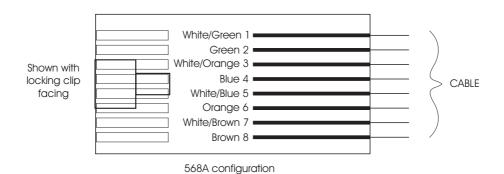
Ensure that the RJ45 connectors are suited to the cable used (solid or stranded) and that the correct crimp tool is used.
